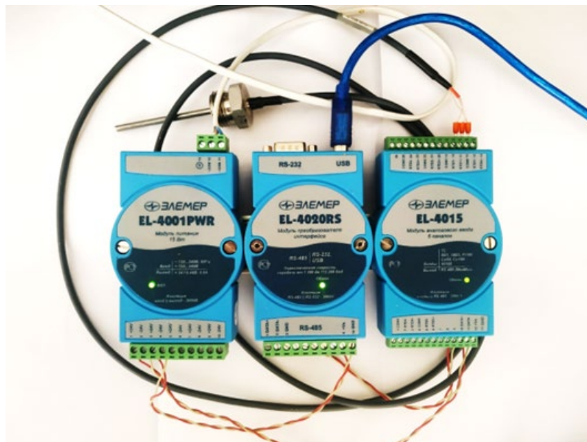
Figure 2. Assembled temperature control system
